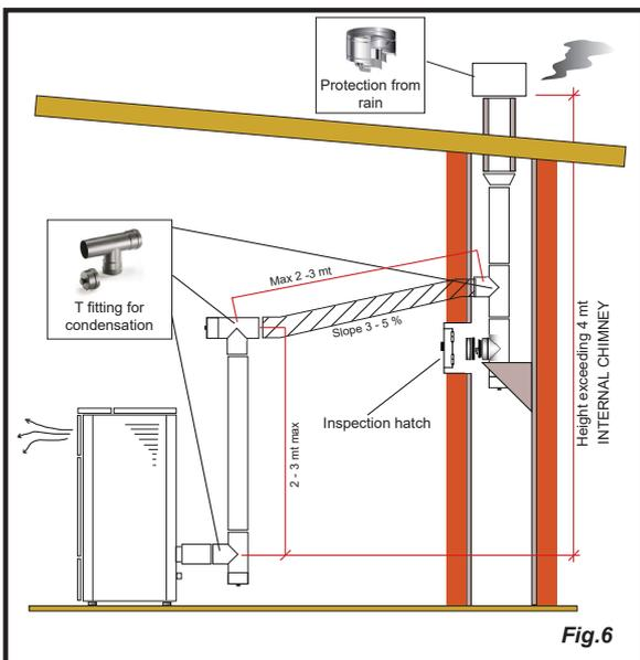
This type of installation (See Fig.6) requires a horizontal section to connect to a pre-existing chimney pot.
