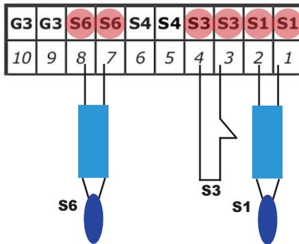
**Connections for diagram 3 (boiler + buffer tank)**
