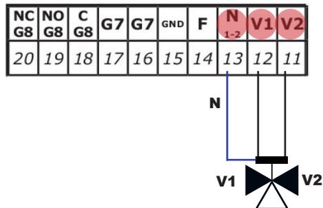
**Connections for home automation and gas boiler**
