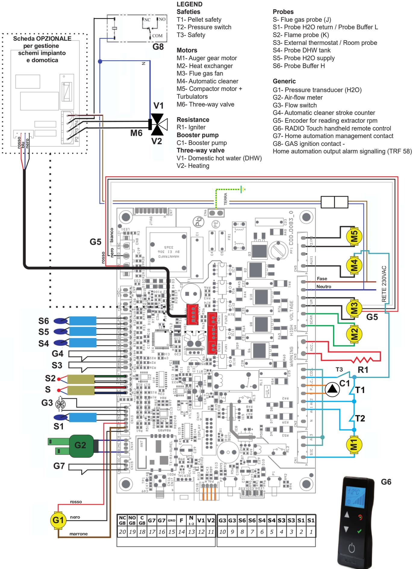
**Connections for hydraulic diagrams**
