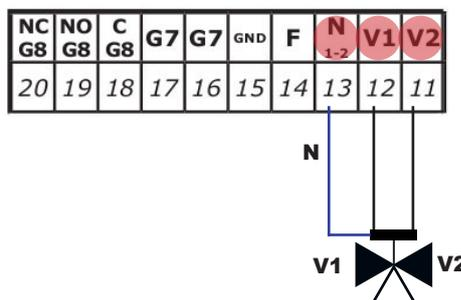
**Connections for diagram 1 (boiler)**
