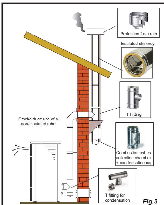
It is possible to use an existing chimney or a shaft via ducting. For this type of installation the standards on ducted smoke evacuation systems must be complied with. In the lower part of the chimney pot, inside the home, there is a "T" type fitting installed; externally there is another one installed, so that the outside section can be inspected.
