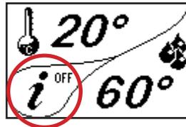
In this condition, by touching the CONFIRM button you can read the detail of the warning: “doors and ash pan open”. If the combustion chamber door, the pellet hopper lid and / or the ash drawer are not closed within 1 minute, the stove switches off signaling ALARM 07. Opening the doors also interrupts the automatic cleaning phase of the brazier. In the event of a prolonged interruption of the cleaning phase, ALARM 19 may appear.
