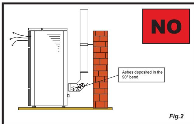
It is prohibited to install a 90° bend for the initial segment, since the ashes would quickly obstruct smoke passage, causing draught problems in the appliance. (See Fig. 2)
